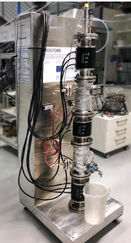
ERT reactor for characterizing gas distribution in bubble column.
